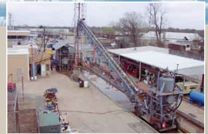
Fig 2: Tulsa University flow loop used for qualification test.
