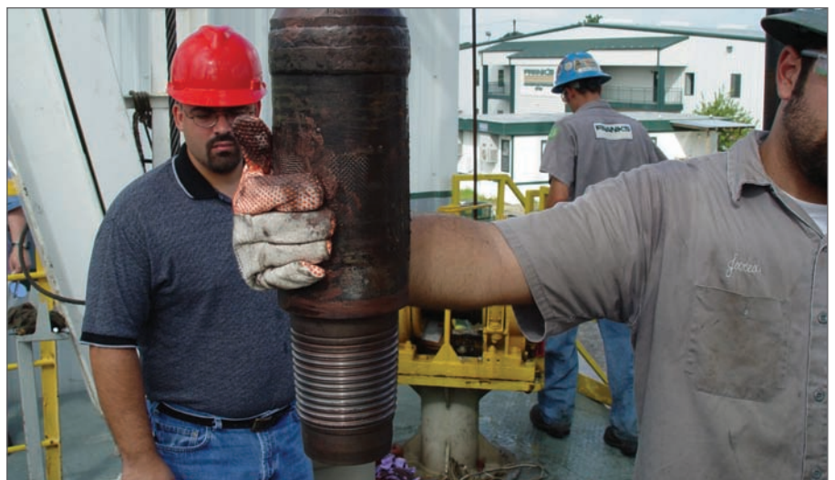
VAM Express allows for quick make-up, with 5-6 turns from stab-in to full make-up.
